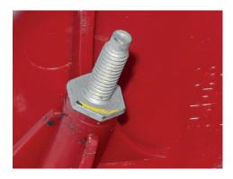
The lack of a vulcanised fibre disc can cause corrosion on the vehicle.
