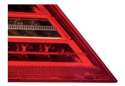
After the stress crack test has been carried out, the lens of the copy rear light shows numerous cracks and in some places it had come completely away from the housing.
