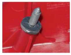
The vulcanised fibre disc protects the vehicle from corrosion.
