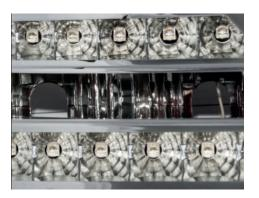
Sink marks and deformations in the reflector surfaces prevent a perfect light distribution.
