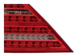
The ULO Original part does not show any changes after the stress crack test.
